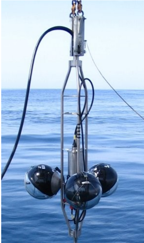
Storey 21 (3 “Acoustic Modules”, 6 sensors in total)
