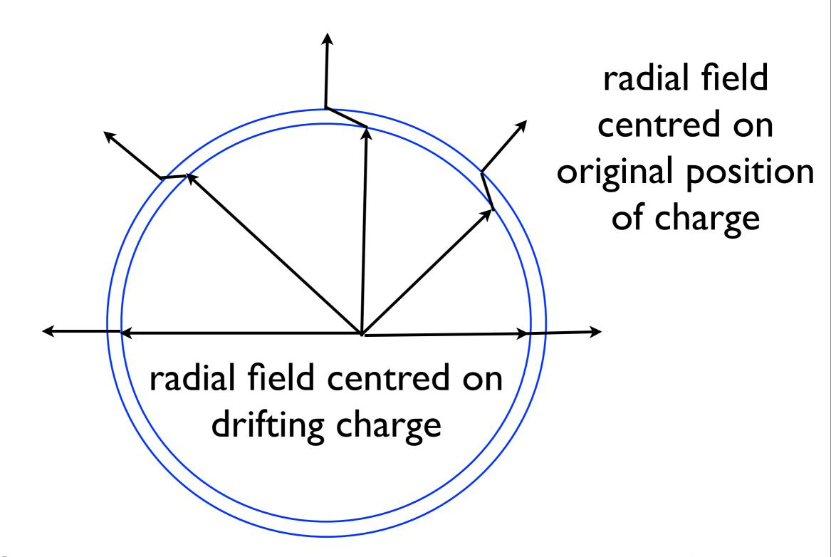
Charge initially at rest, given small impulse  $\Delta V$
