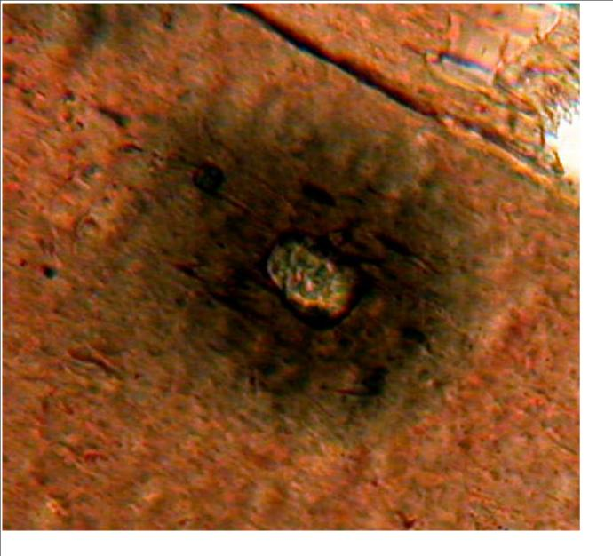
Explanation for pleochroic halos observed in many minerals around radioactive inclusions.
