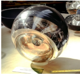
Optical Module (10" PMT in 17" glass sphere) photon detection
